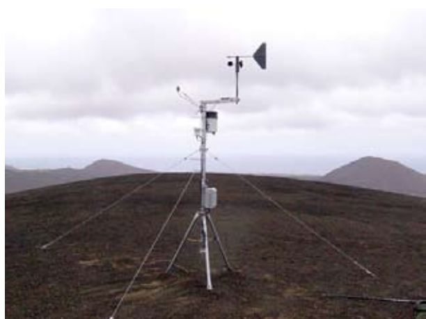
Figure 3. Weather station on Sisters Peak Ascension Island. We have also collated Global Circulation Model predictions and historical climate data to characterise past, present and future climate on Ascension.
